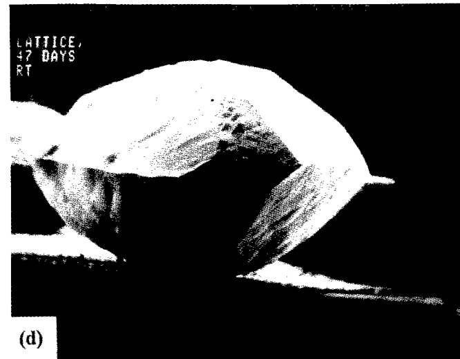
Fig. 5. The samples in (a) and (c) are shown normal to the Z-axis; the samples in (b) and (d) are shown normal to the +X-axis. (a) Etched in 40%/60% (see text) for 2 days at 80°C. (b) Same as (a). (c) Etched in Lattice Etch™ for 47 days at room temperature. (d) Same as (c). Note the similarities between 5(a) & (b) and 4(a) & (b).
